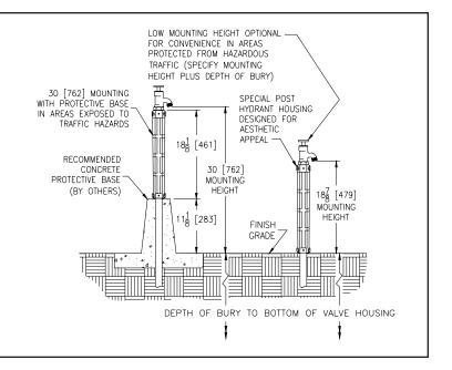
**NOTE:** For ground, post, and yard hydrant installations that involve the use of a drain port, it is recommended that gravel be placed around the drain port to allow a flow path for the drained water to evacuate.
