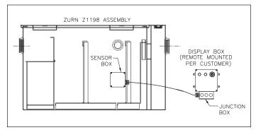
Zurn oil interceptors with oil level sensors are efficient appliances designed to separate oil from water.
