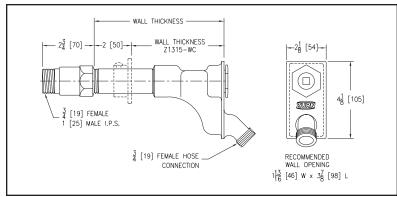
**ENGINEERING SPECIFICATION:** ZURN Z1315 Exposed, non-freeze wall hydrant with bronze casing, all bronze interior parts, non-turning operating rod with free-floating compression closure valve, replaceable bronze seat and seat washer, and combination 3/4" [19 mm] female or 1" [25 mm] male straight IP inlet. Complete with operating key.
