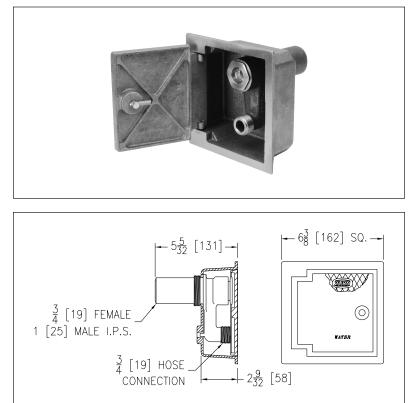
**ENGINEERING SPECIFICATION:** ZURN Z1335 Encased flush wall hydrant, for moderate climate and interior wall installation. Complete with all bronze interior parts, non-turning operating coupling with free-floating compression closure valve and replaceable bronze seat and seat washer, and 3/4" [19 mm] female IP inlet. Nickel bronze box and hinged cover with operating key lock and "WATER" cast on cover.
