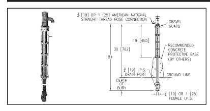
**ENGINEERING SPECIFICATION:** ZURN Z1385 Exposed, non-freeze post hydrant. Complete with bronze casing and cast aluminum casing guard, all bronze interior parts, bronze seat and replaceable seat washer, and non-turning operating rod with free-floating compression closure valve with 3/4" [19 mm] or 1" [25 mm] connection. Operating key included. Hydrant is equipped with a tapped 1/4" [6 mm] drain port in valve housing.
