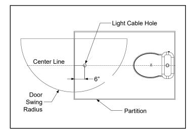
When installing the ceiling mount bracket, it is very important to ensure that the arrow is pointing toward the inside of the stall, perpendicular to the stall door. In most cases, the arrow should be pointing directly towards the water closet. In some different stall configurations, such as handicapped/ADA stalls, the arrow may not point directly towards the water closet.
