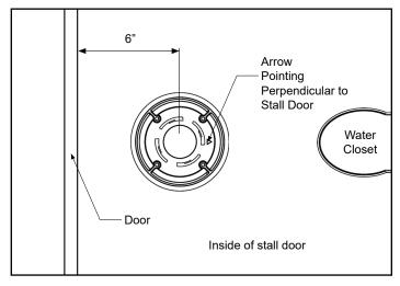
Each component that makes up an occupancy light has a small triangle. This triangle is a arrow that marks the direction of the sensor beam. The arrow should always point towards the inside of the stall that the light is being installed for.
