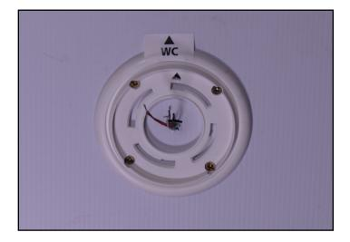
It is crucial that the cables you install are longer than the extension tube that is being used. Ideally the length of the wires should be 4 inches longer than the extension tube to make the installation easier when connecting to the power block.
