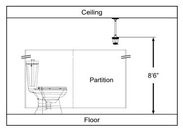
\* Zurn Smart Occupancy Light should be mounted at a max 8'6" feet above the floor, either directly to the ceiling or using a Zurn Smart Occupancy Light Mount - Extension Pole.
