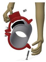
4. Tighten nuts alternately and equally until the outlet housing contacts the pipe, metal to metal. Keep bolt pad gaps equal on both sides. Torque nuts according to the Required Torque Table.
