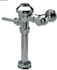
back pressure vacuum breaker, one-piece hex coupling nut, adjustable tailpiece, spud coupling, and flange for top spud connection. Control stop has internal siphonquard protection, vandal-resistant stop cap, sweat solder kit, and a cast wall flange with setscrew. Internal seals are made of chloramine resistant materials.
