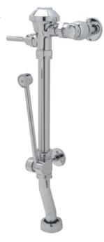
hex coupling nut, adjustable tailpiece, spud coupling and flange for top spud connection. Control stop has internal siphon-guard protection, vandal-resistant stop cap, sweat solder kit, and a cast wall flange with setscrew. Internal seals are made of chloramine resistant materials.
