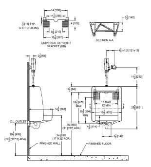
These dimensions and specifications are subject to change without notice. Fixture dimensions meet ANSI/ASME standard A112.19.2 and CAN/CSA B45 requirements.
