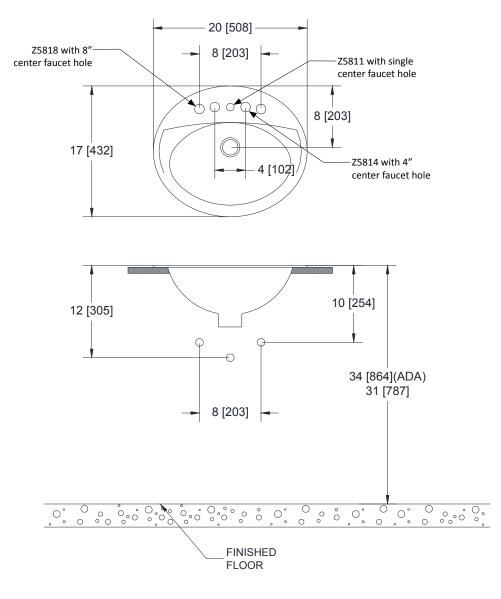
Fixture dimensions meet ASME A112.19.1 / CSA B45.2 requirements.
