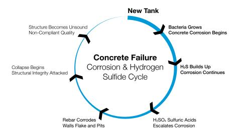
Hydrogen sulfide is not only harmful, it is a major contributor to untreated concrete and steel interceptor failure, as aerobic bacteria converts H<sub>2</sub>S to sulfuric acid which is highly corrosive.
