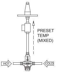
ZW3870XLTF3PORT (1 Hot in, 1 Cold in, 1 Mixed out)ZW3870XLTF-4P4PORT (1 Hot in, 1 Cold in, 1 Cold out, 1 Mixed out.)
