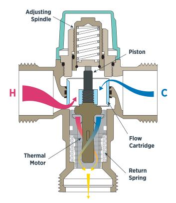
When mixed water is too cold, flow cartridge moves up, allowing more hot water to enter
