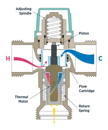
When mixed water is too hot, flow cartridge moves down, allowing more cold water to enter
