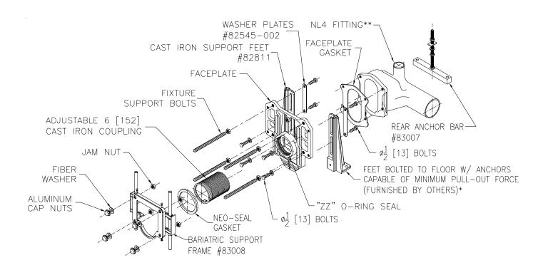
\*Carrier foot anchors must be able to withstand a pull-out force of 335 Lb.[152 kg.]. Calculated value, no safety factor applied.
