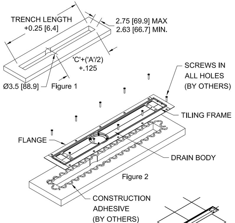
2. Set drain body into slot and ensure membrane flange lays flat on floor. Attach body to floor with construction adhesive and corrosion resistant #8 countersunk screws (provided by others). If installed in metal floor, flooring must be countersunk. Ensure all body lockdown holes are utilized, taking care to not warp flange when tightening screws (Figure 2). Wipe away all excess adhesive and ensure body and floor are clear of debris.
