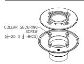
Step 4: Install clamping collar.
