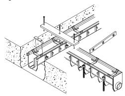
Typically, a trench system is assembled from the outlet on back. Starting with the deepest section or catch basin, set the first channel utilizing Perma-Trench's unique anchoring system. Integral rebar clips are located along the length of each trench drain and catch basin for easy attachment to #4 rebar stakes. Simply align the rebar stakes with the trench drain and drive them into the ground for positive anchoring. Attach the trench drain to the rebar stakes with the hardware provided.
