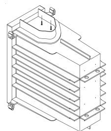
3. Attach the incoming trench section with the hardware provided to complete the connection. Silicone adhesive may be used to keep debris from building up in the connection.
