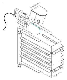
2. Cut inlet adaptor to the correct depth and place as shown below. Drill 4 holes evenly spaced and thread screws through the adaptor into the catch basin.
