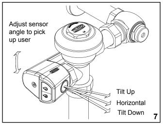
7. Loosen handle nut, aim sensor at desired tilt angle (horizontal, tilt up, or tilt down), hold in place and tighten handle nut
