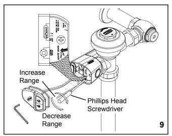
Adjust feature settings as desired. The sensor range is factory set to 48". If adjustment is necessary, use a phillips head screwdriver and turn GENTLY. SEE SENSOR RANGE ADJUSTMENT. Replace electronics access cover and tighten securely with vandal-resistant hex wrench.
