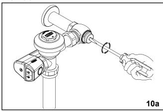
Before the supply water is turned on, be sure all stop valves to the flush valves are closed off tight. The stop valves can be opened and closed by using the adjusting screw located at the center of the stop valve cap (shown in 10a), behind the adjusting screw cover if already installed. Stop valve adjustments can only be made by using the adjusting screw. It is not necessary to remove the stop valve cap when making adjustments. If for any reason it becomes necessary to remove the stop valve.
