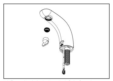
1.3. Ensure that slot in plastic washer is facing forward.
