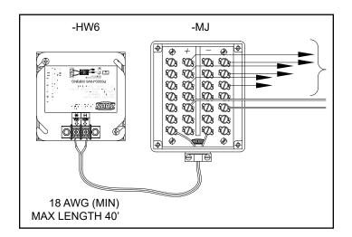
2.3b. Optional HW6 (Hardwired 6V) version: Connect supplied inline connector and hardwire adapter. When securing the CWB wires to the screw terminals on HW6 unit, the BLACK WITH DASHED MARKINGS should be connected to the Positive (+) terminal, and the SOLID BLACK wire should be connected to the Negative (-) terminal.
