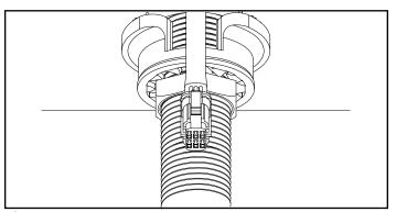
Take care passing sensor cable through hole. Cable passes through front of plastic mounting washer
