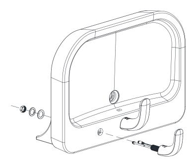
For ease of installion, lay basin on its back. Install the soap spout on right or left soap hole as applicable. Refer to soap dispenser installation guide for details.
