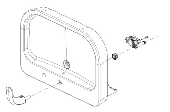
For ease of installion, lay basin on its back. Refer to faucet installation guide for details.
