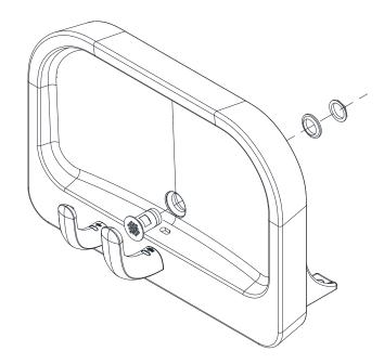
For ease of installion, lay basin on its back. Place grid drain into drainage opening. Fasten washer and nut from underside of basin.
