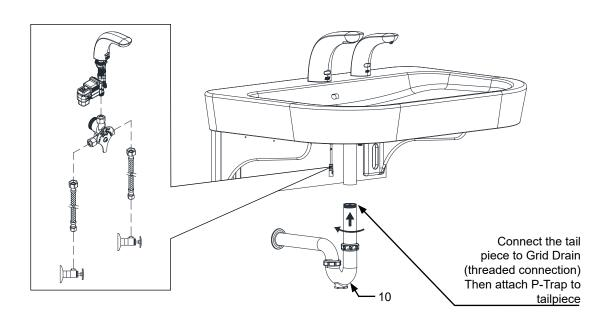
Adjust the tail piece base on drain outlet on the wall.
