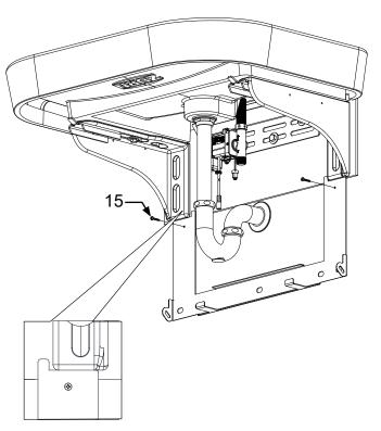
Align wall bracket as shown and install coarse screw on each side. Mark the slots in the wall bracket on the wall.
