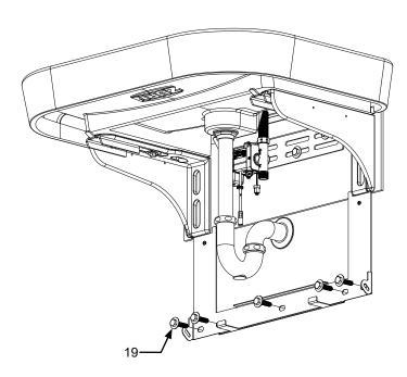
• Re-install wall bracket with coarse screws in previous location. Then, fasten the wall bracket with 3/8" bolts through each holes and into the toggle bolts.
