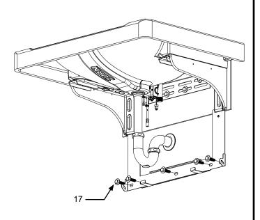
Re-install wall bracket with coarse screws in previous ٠ location. Then, fasten the wall bracket with 3/8" bolts through each holes and into the toggle bolts.
