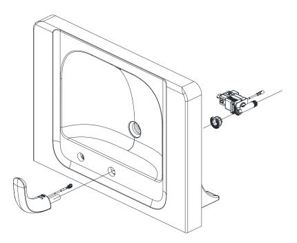
Note: Installing the P-trap outlet lower than 19.5" from finished floor will prevent the vandal shroud from being installed.
