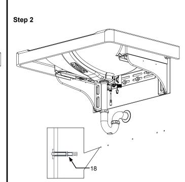
Remove the wall bracket and drill 3/4" holes into the • center of the holes previously marked. (Note: For installation with carrier, do NOT drill the two outside holes. For retrofit applications, the two outside holes are recommended.) Ensure that wall studs are not immediately behind the marked hole locations prior to drilling.
