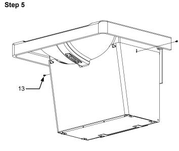
• Rotate the shroud up to the basin until the threaded hole in the L-bracket in visible through the slot in the shroud. Then, install the screw shown, and repeat for the other side.
