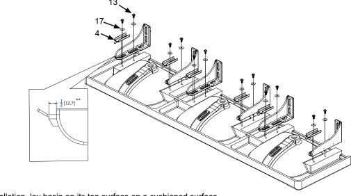
For ease of installation, lay basin on its top surface on a cushioned surface. Install hanger brackets 1/2 inch from front face of L-bracket as shown.\*\* Use socket wrench to torque the screws (approximately 4-5 complete turns bottom out approximately 5 ft-lbs of torque).
