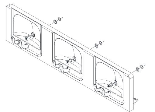
For ease of installation, lay basin on its back. Place grid draininto drainage opening. Fasten washer and nut from underside of basin.
