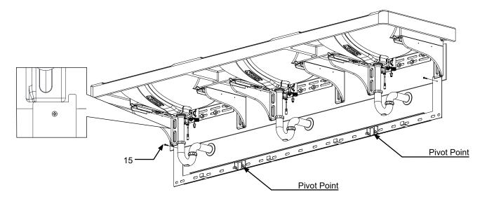
• Align wall bracket as shown and install coarse screw on each side. Mark the slots in the wall bracket on the wall. (Note: Anchors and bolts location can be flexible base on on-site wall studs location) (Note: A minimum of one anchor next to each pivot point is required to prevent excessive flexing when shroud is in fully open position)
