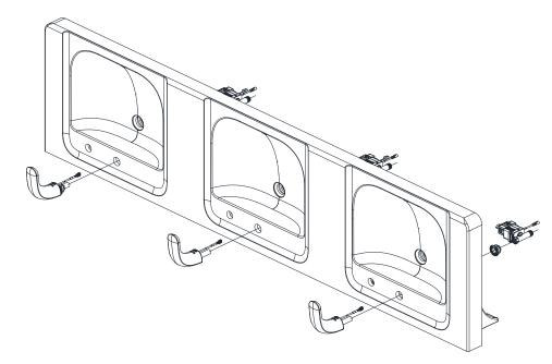
For ease of installation, lay basin on its back. Refer to faucet installation guide for details.
