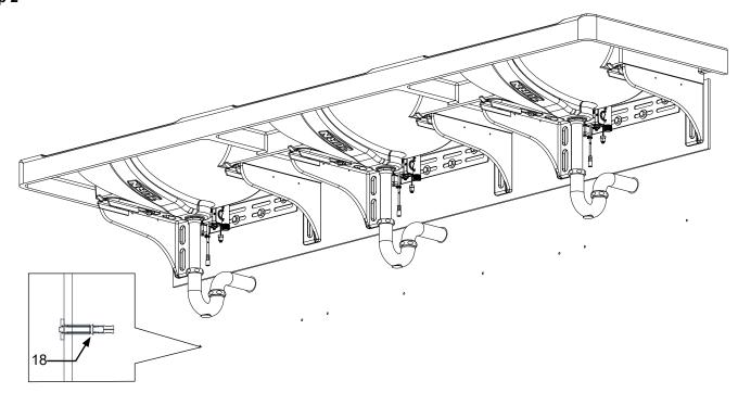
• Remove the wall bracket and drill 3/4" holes into the center of the holes previously marked. Ensure that wall studs are not immediately behind the marked hole locations prior to drilling.
