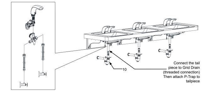
Adjust the tail piece base on drain outlet on the wall.
