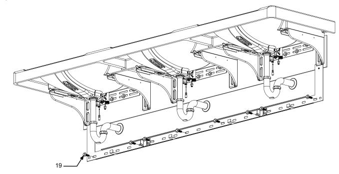
• Re-install wall bracket with coarse screws in previous location. Then, fasten the wall bracket with 3/8" bolts through each holes and into the toggle bolts.
