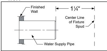
3. Measure distance from finished wall to first thread of sweat solder adapter. If necessary, cut chrome cover tube this length.
