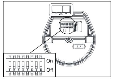
4. Adjust the battery detection function by manipulating DIP switches #8 according to the table provided below:
