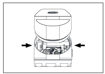
3. Adjust the courtesy flush interval by manipulating DIP switches #2 and #3 according to the table provided below:
