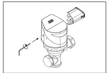
3. Slide the battery tray back into the valve head and apply firm pressure. Turn the 3/32" Allen Wrench clockwise to tighten the battery tray screw to a dead-stop and ensure the battery tray is flush with the valve head.
