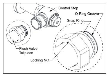
Prior to attaching flush valve tailpiece to control stop, inspect and verify that the O-ring seal is located within the O-ring groove at the tailpiece. Ensure that the locking nut and locking snap ring are also present on the tailpiece.
