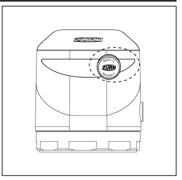
Note: To ensure proper functionality, make sure the calibration distance in water closet applications prevents the sensor from detecting the stall door. Verify this by closing the door for 10 seconds, then opening it. If the flush valve doesn't activate, the calibration distance is suitable. Otherwise, recalibrate to a closer distance using the magnet.
