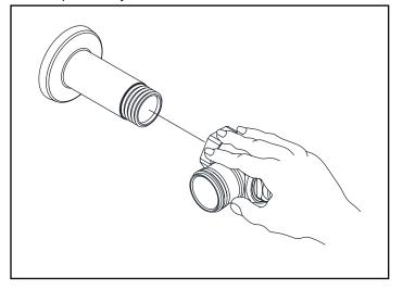
2. Slide threaded sweat solder adapter onto water supply pipe until shoulder stops on end of pipe. Then sweat-solder the adapter to water supply pipe.
