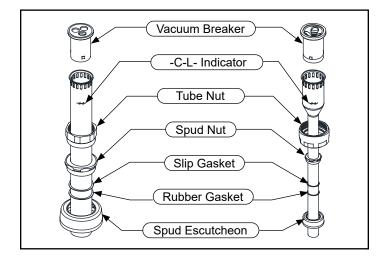
Determine the length of vacuum breaker tube required to join the flush valve and fixture spud, and cut if necessary.
