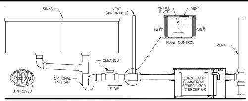
Zurn Light Commercial Series Grease Interceptors GT2700 consist of a interceptor rated at ( ) gpm and a properly sized flow control fitting.
