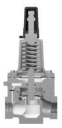
**Drip Tight Closing Operation**The compressed spring forces the plunger on the seat creating a drip tight seal.
