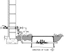
**C.** If you are using a Double Check Backflow Preventer in a meter box, install the outlet tailpiece in the vertical down position.
