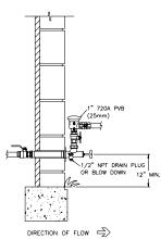
A. If you are using a Pressure Vacuum Breaker, install the Winterizer with the outlet tailpiece facing upwards vertically.
