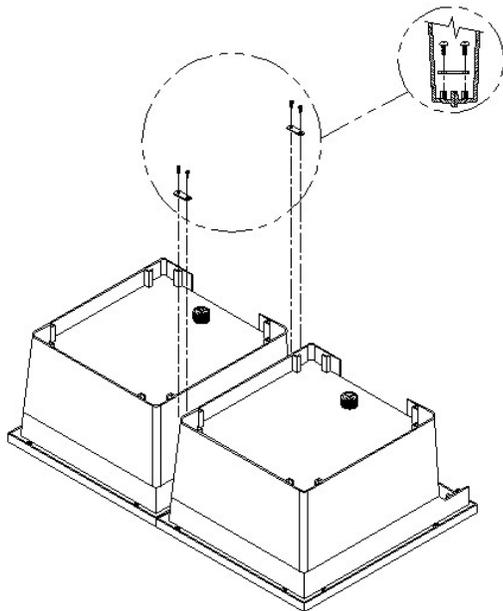
Attach the plastic connector to the four towel bar lugs on the underside of the sinks using the four screws provided.
