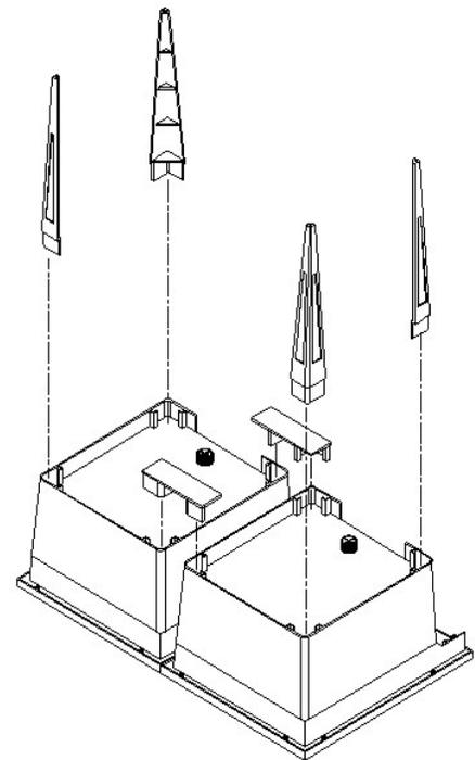
Insert the metal connector brackets into the leg slots as shown. Tap gently with a hammer if the fit is tight. Insert the four legs in the four remaining leg slots.
