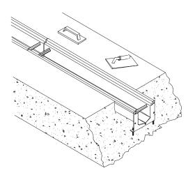
Allow for concrete shrinkage during finish troweling so that the top surface of the trench drain doesn't protrude from the floor surface after concrete has cured.
