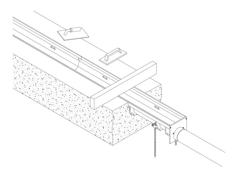
\*It is recommended to pour concrete the same day the trench is set. Failure to do so could cause trench cracking when subjected to temperature variations.
