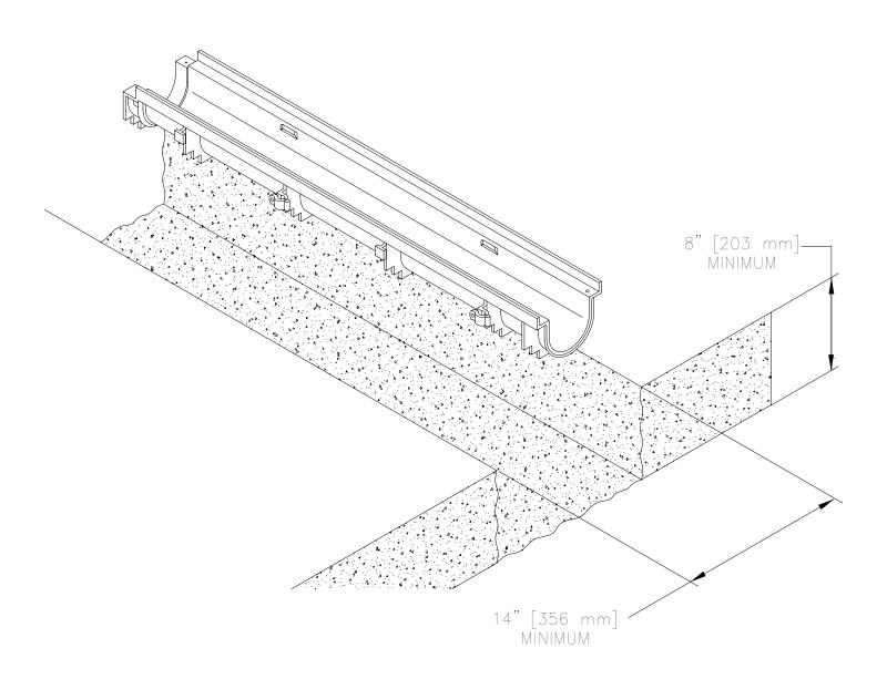
Trench excavation must be 4 [102] greater than the trench depth and a minimum width of 14 [356]. Soft and/or shifting soil substrates may cause cracking of the concrete and consequent movement of the trench. It is critical that the concrete be poured on an adequate foundation.
