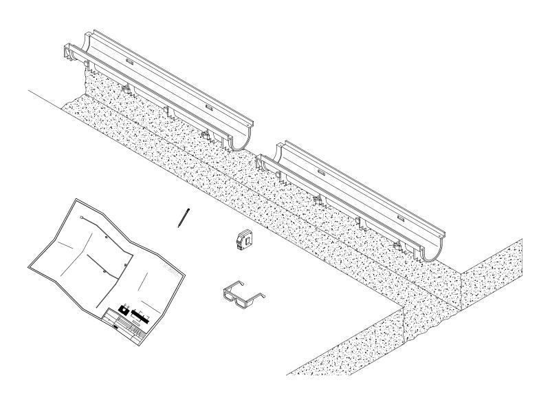
Upon completion of the trench excavation, the channels should be placed in order alongside the excavation and according to the job layout. Grates are not installed at this time.
