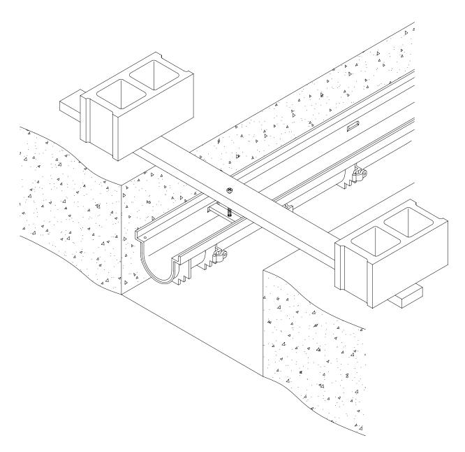
An alternative means of installation is to suspend the trench drain as shown. Wooden braces to hang the trench run can be attached to the drain body through the grate lock down bars as illustrated above.
