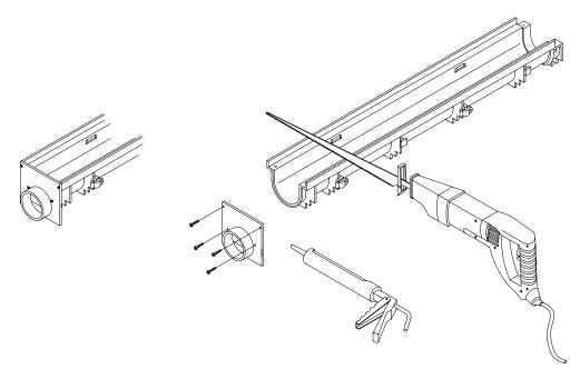
A bottom outlet is attached to the bottom side of the trench drain with provided screws and a silicone caulk or a construction adhesive if desired as shown below. A hole saw can be used to cut the appropriate size hole through the bottom of the trench.
