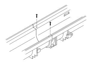
Assembling the trench run is easy using 'Flo-Thru" mechanical interlocking joints. Simply align the two mating ends of the trench sections and fasten with the hardware fasteners provided. A silicone caulk, or a construction adhesive, such as Liquid Nails, is recommended to be used at each joint as a sealer.
