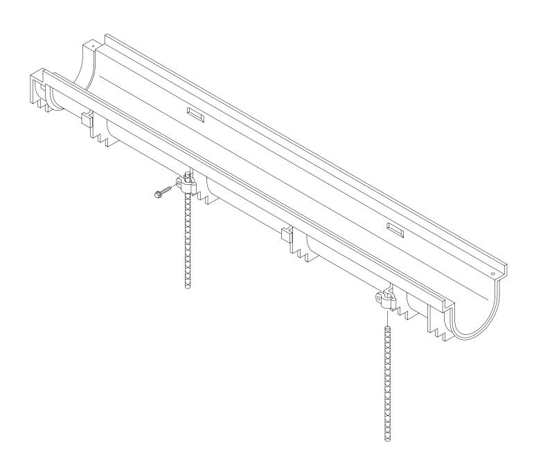
Typically, a trench system is assembled from the outlet on back. Starting with the last section or catch basin, set the first channel utilizing Flo-Thru's unique integral Rebar Clip anchoring system.Rebar clips are used on both sides of the length of each trench drain for easy attachment to 3/8 [10] rebar stakes. Simply place through rebar clips and drive the stakes into the ground for positive anchoring. Attach the trench drain to the rebar stakes with the hardware provided.
