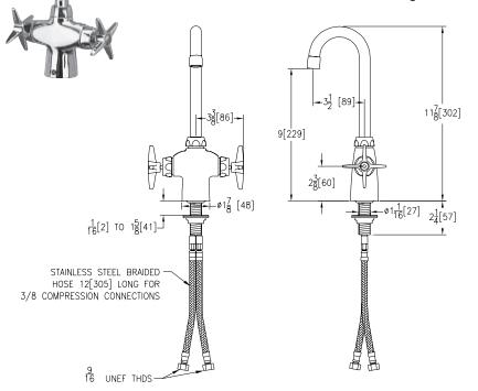
Zurn Lead Compliant\* "XL" products are a line of durable, high quality brass faucets and fixtures that are designed and manufactured to comply with state laws and local codes that mandate lead content levels. Zurn "XL" products are manufactured with \*not more than 0.25% lead content when used with respect to wetted surfaces of pipes and pipe fittings, plumbing fitting and fixtures: California Health & Safety Code § 116875; Vermont 9 VCA § 2470h
