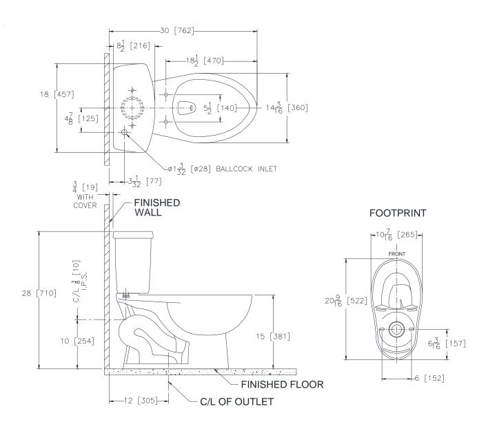
Fixture dimensions meet ANSI/ASME standard A112.19.2 and CAN/CSA B45 requirements.
