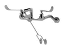
Engineering Specification: Zurn AquaSpec® Z842D6-LSI-LVB-PE-5XT Polished chrome-plated cast brass 8" [203mm] clinical service sink faucet with quarter-turn ceramic disc cartridges, 2 1/2" [64mm] long swivel inlets (with integral stops) providing adjustable centers from 3" [76mm] to 13" [330mm] and a 7 1/8" [181mm] centerline cast brass, plain end spout with a pail hook and a forked bottom brace. Unit is furnished with 6" [152mm] vandal-resistant color-coded metal wrist blade handles.
