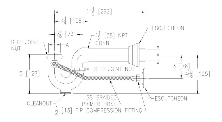
A - Pipe Size 1-1/2 [38] **ENGINEERING SPECIFICATION:** ZURN Z1021 Water Saver Trap Primer, chrome plated polished cast brass body with cleanout, ground joint elbow with 1-1/2 [38] NPT outlet, 1-1/2 [38] slip nuts and washers, and reducing washer for 1-1/4 [32] sink tail piece hookup, escutcheons and stainless steel braided primer hose with 1/2 [13] FIP compression fittings.
