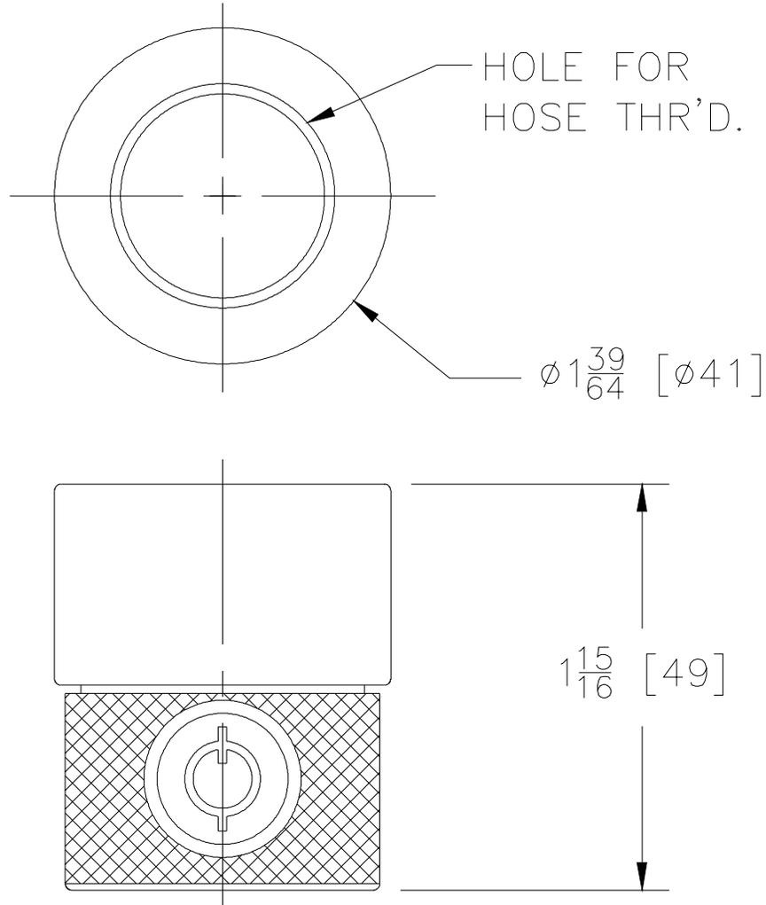
**ENGINEERING SPECIFICATION:** Z1399-HG Brass hose bibb lock with key operated lock/un-lock feature for 3/4 [19] hose thread connection.
