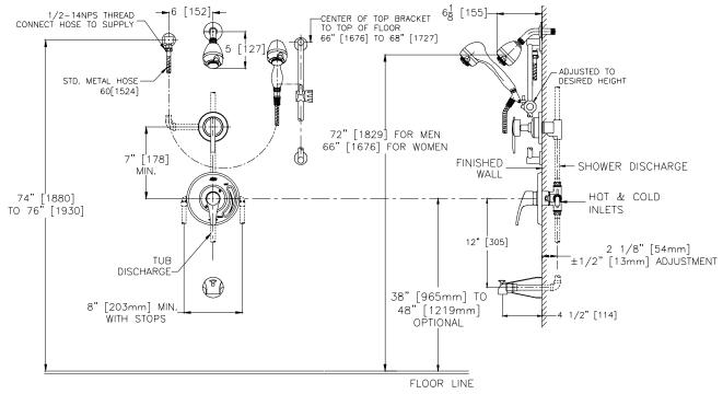
Note: All dimensions are for reference only. Do not use for pre-plumbing. Parts shown as hidden lines are supplied by others.
