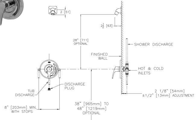
Note: All dimensions are for reference only. Do not use for pre-plumbing. Parts shown as hidden lines are supplied by others.
