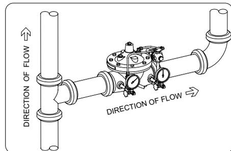
**Caution:** The recommended installation orientation for ACVs is horizontal, with the valve cover up. 6" and larger valves should only be installed horizontally, with the valve cover up, due to the difficulty of properly bleeding air out of the cover and performing maintenance on valves installed in the vertical orientation.
