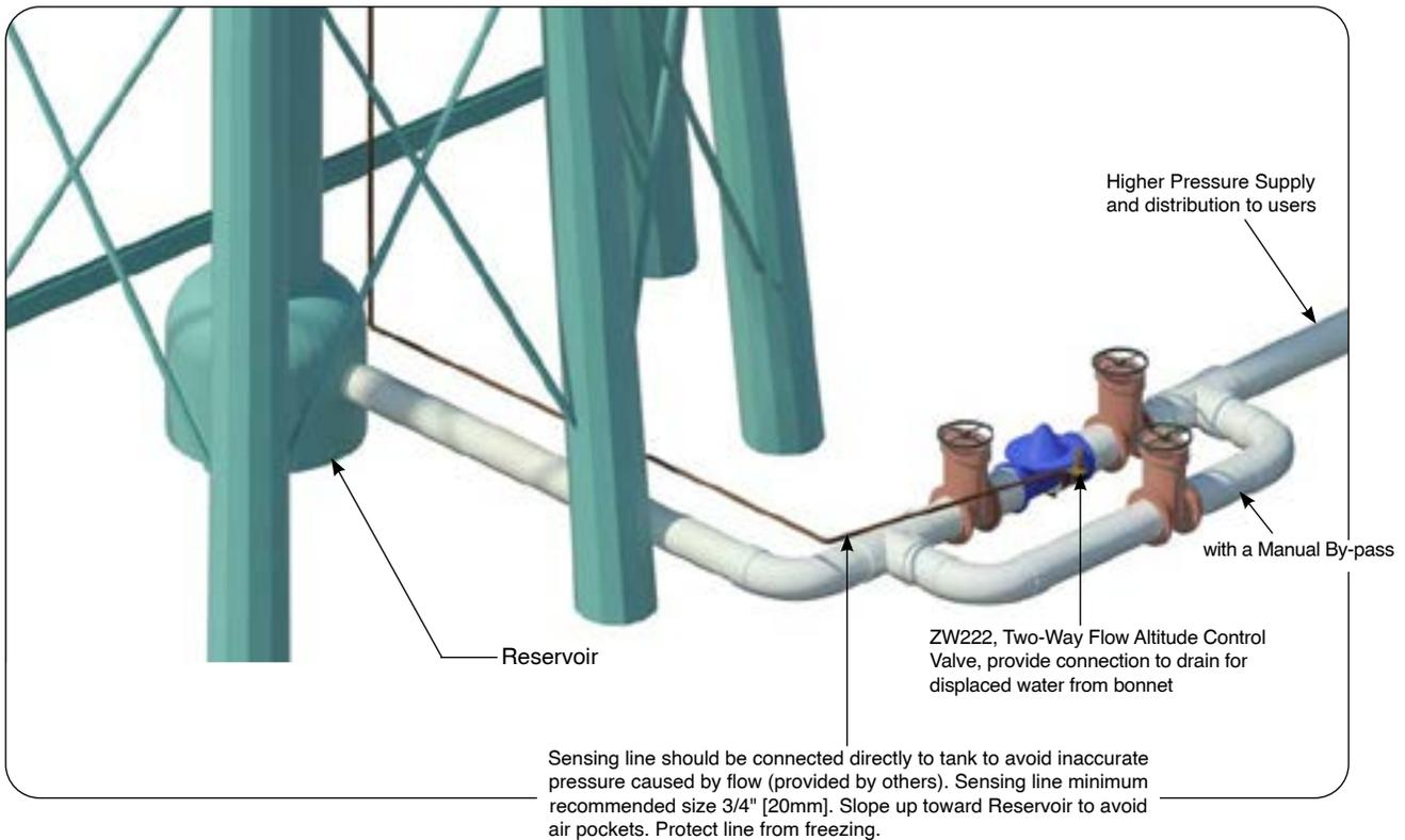
**Caution:** The recommended installation orientation for ACVs is horizontal, with the valve cover up. 6" and larger valves should only be installed horizontally, with the valve cover up, due to the difficulty of properly bleeding air out of the cover and performing maintenance on valves installed in the vertical orientation.
