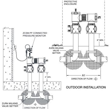
INDOOR INSTALLATION (450STR with ZCSM-PF Connected Pressure Monitor Accessory)
