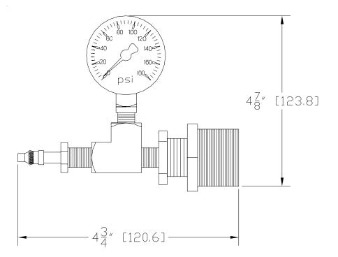
**Engineering Specification:** Zurn® air pressure test kit. Brass fittings with test gauge and schrader valve. Complete with 1" or 1-1/4" MNPT brass adatpter to adapt to Zurn Radiant heating manifolds. Pressure rating up to 180 PSI.
