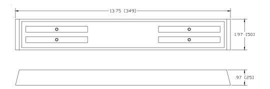
**Engineering Specification:** Zurn Ground Sensor for slab sensing. Designed for slab embedding. Sensor has both moisture and temperature sensors. Unit has a built-in 2W heating element. Sensor can measure temperature only or temperature and moisture.
