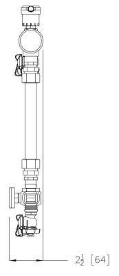
**Engineering Specification:** Zurn Pressure By-Pass Kit. Adjustable by-pass valve from 0 - 19 feet of head. By-Pass loop using 3/4" ZurnPEX® tubing. Kit shall also include air vent, fill/drain valves, and thermometer.
