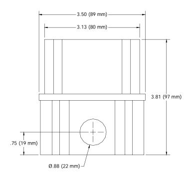
**Engineering Specification:** The Zurn PEX<sup>®</sup> Snow and Ice Melt Socket. The QHSIS is used to house the Snow and Ice Melt Detector (QHSID). The brass socket should be located directly in between two pieces of Zurn PEX tubing in the snow and ice melt slab. Also included is a mounting plate and a plastic plug, which is the same thickness as the QHSID sensor.
