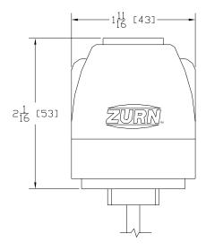
**Engineering Specification:** Zurn Zone Valve Actuator allows for zone valve control. Unit operates on 24VAC, 2W. Complete with pop-up indicator. Connects to zone valve with threaded adapter and actuator is snap on/off to adapter.
