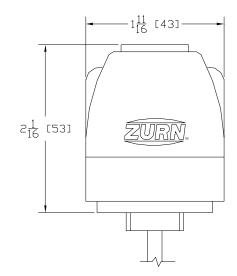
**Engineering Specification:** Zurn Zone Valve Actuator with end switch allows for zone valve control. Unit operates on 24VAC, 2W. Complete with pop-up indicator. Connects to zone valve with threaded adapter and actuator is snap on/off to adapter.
