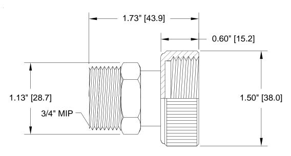
Engineering Specification: ZurnPEX® XL-Low Lead Brass 1" Swivel x 3/4" MIP QickPort® Connection. The QQTFC45GX is used to connect FIP to the QickPort® manifold. Manufactured from EcoBrass®. These fittings are listed by NSF as complying with the following standards: NSF/ANSI Standard 61 including Annex G.
