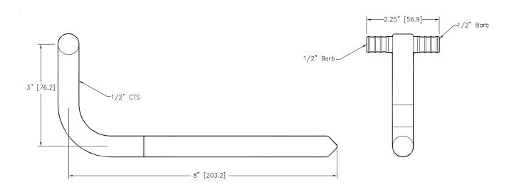
**Engineering Specification:** ZurnPEX<sup>®</sup> 1/2" Copper Stubout Tee Elbow. The QSTUBLXXT3 elbow tee is used in conjunction with PEX tubing. QSTUBLXXT3 is ideal for stubouts off of 1/2" ZurnPEX<sup>®</sup> runs. End spun closed allows for system testing before valves or other fittings are installed. Meets NSF® and ASTM requirements.
