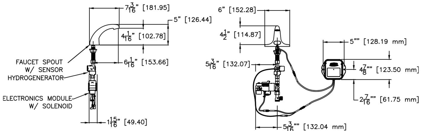
*Note: Endpoint must be installed within a 2' [610] radius of faucet.*
